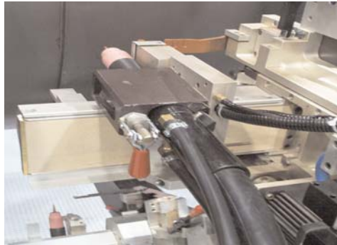
Weldhead with Patented Laser Tracking
